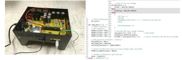
This particular VFD features a power factor correction stage, a functionality required by more and more government regulations. This topology is also known as a boost converter. Software controls are used to control this device to regulate voltage on the DC bus.
