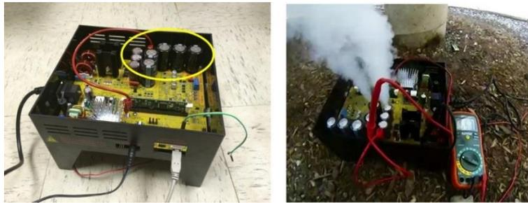
**Figure 2. (Left) Small VFD test kit, (Right) Explosion of VFD test kit caused by minor firmware changes**
